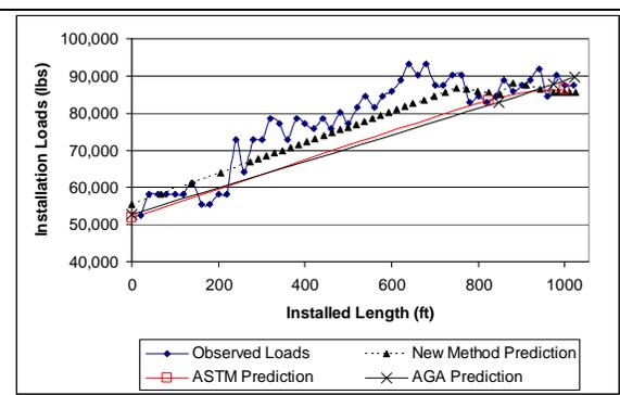
Figure 8. Observed and predicted loads during pullback operations
