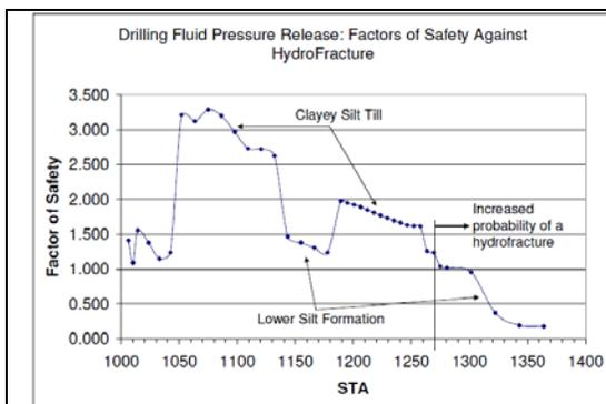
Figure 7. Estimated factor of safety during pilot bore drilling.
